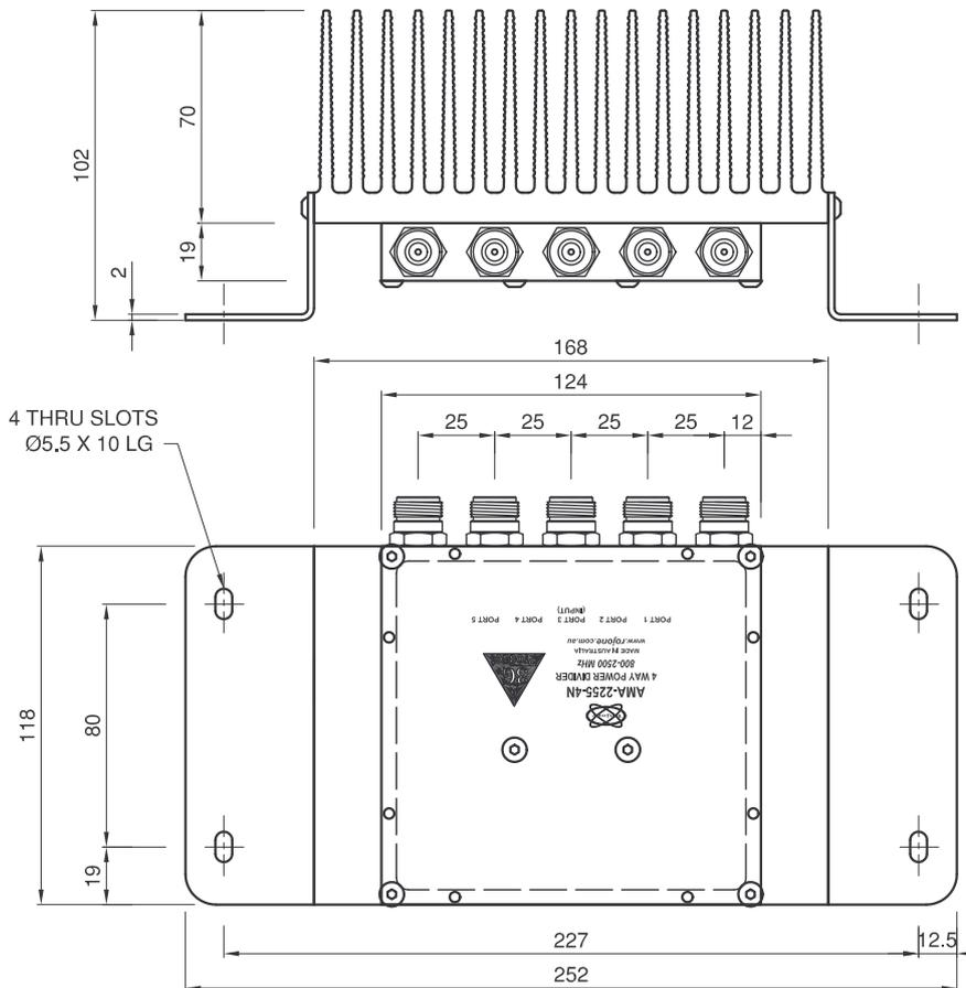
Recommended coupling torque force for N connector 40 to 60 Ncm.
