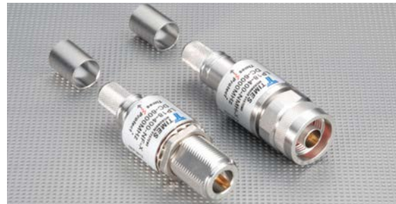
Crimp N Male and Female for LMR-400 with Lightning Protection, DC-6 GHz; 13AL (male), 13FL (female)
