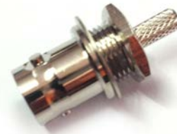
Front mount bulkhead cable jack inserts from front of panel, secure nut at rear of panel.
