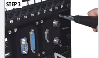
Using a Phillips or Flat screwdriver, install your sub-panels in the master rack panel.
