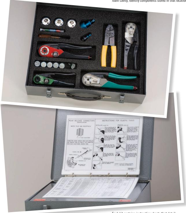
Each kit contains instruction sheets that detail application and explain how each tool is used. Tool selection sheets further add to the ease of kit use by referencing tool requirements for each connector series covered by the kit. All reference sheets in each kit are coated to protect against the elements.
