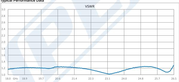
Click the following link (or enter part number in "SEARCH" on website) to obtain additional part information including price, inventory and certifications: WR-42 Waveguide 40 dB Crossquide Coupler, UG-595/U Square Cover Flange, SMA Female Coupled Port, 18 GHz to 26.5 GHz, Bronze PEWCT1050
