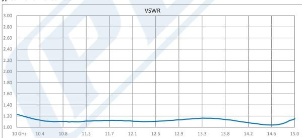
Click the following link (or enter part number in "SEARCH" on website) to obtain additional part information including price, inventory and certifications: WR-75 Waveguide Circulator, 10 GHz to 15 GHz, 18 dB min Isolation, Cover Flange, Aluminum PEWCR1002
