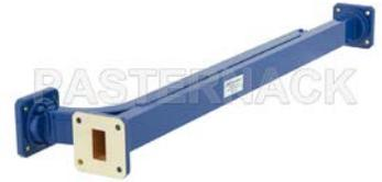
WR-75 20 dB Directional Waveguide Broadwall Coupler, Square Cover Flange, E-Plane Coupled Port, 10 GHz to 15 GHz
