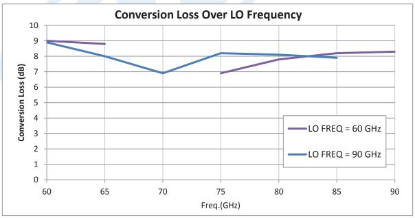
Click the following link (or enter part number in "SEARCH" on website) to obtain additional part information including price, inventory and certifications: Waveguide Mixer Down Converter WR-12 From 60 GHz to 90 GHz, IF From DC to 18 GHz And LO Power of +13 dBm, UG-387/U Flange, E Band PE12D1001
