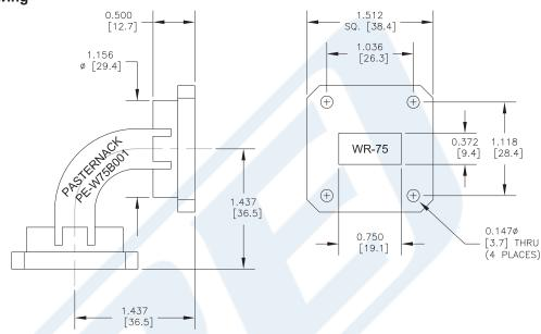
WR-75 Waveguide E-Bend with UG-584/U Flange Operating from 10 GHz to 15 GHz from Pasternack Enterprises has same day shipment for domestic and International orders. Our RF, microwave and millimeter wave products maintain a 99% availability and are part of the broadest selection in the industry.
