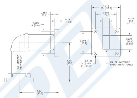
WR-62 Instrumentation Grade Waveguide H-Bend with UG-419/U Flange Operating from 12.4 GHz to 18 GHz from Pasternack Enterprises has same day shipment for domestic and International orders. Our RF, microwave and millimeter wave products maintain a 99% availability and are part of the broadest selection in the industry.
