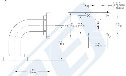
WR-62 Waveguide H-Bend with UG-419/U Flange Operating from 12.4 GHz to 18 GHz from Pasternack Enterprises has same day shipment for domestic and International orders. Our RF, microwave and millimeter wave products maintain a 99% availability and are part of the broadest selection in the industry.
