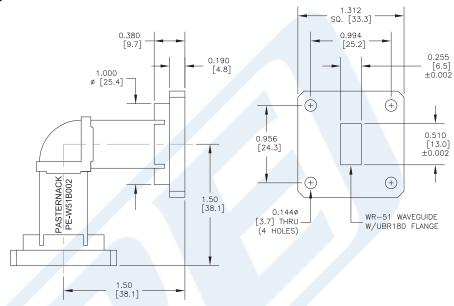
WR-51 Instrumentation Grade Waveguide H-Bend with R180 Flange Operating from 15 GHz to 22 GHz from Pasternack Enterprises has same day shipment for domestic and International orders. Our RF, microwave and millimeter wave products maintain a 99% availability and are part of the broadest selection in the industry.
