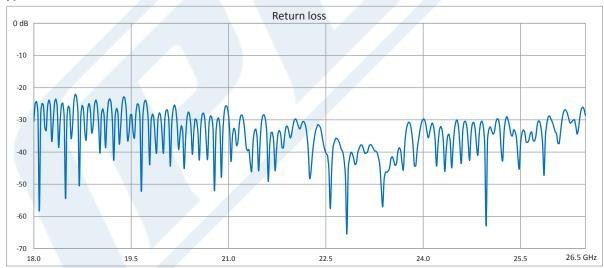
Click the following link (or enter part number in "SEARCH" on website) to obtain additional part information including price, inventory and certifications: WR-42 Seamless Flexible Waveguide 36 Inch, UG-595/U Square Cover Flange Operating From 18 GHz to 26.5 GHz PE-W42SF005-36
