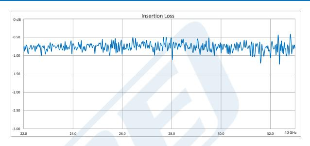
WR-34 Seamless Flexible Waveguide 24 Inch, UG-1530/U Square Cover Flange Operating From 22 GHz to 33 GHz from Pasternack Enterprises has same day shipment for domestic and International orders. Our RF, microwave and millimeter wave products maintain a 99.4% availability and are part of the broadest selection in the industry.
