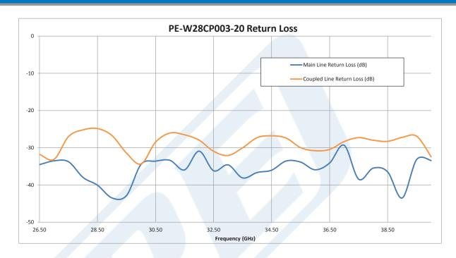
WR-28 20 dB Directional Waveguide Coupler With UG-599/U Flange and E-Plane Coupled Port From 26.5 GHz to 40 GHz Ka Band from Pasternack Enterprises has same day shipment for domestic and International orders. Our RF, microwave and millimeter wave products maintain a 99% availability and are part of the broadest selection in the industry.
