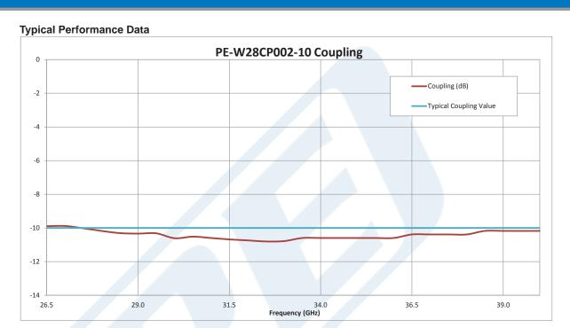
Click the following link (or enter part number in "SEARCH" on website) to obtain additional part information including price, inventory and certifications: WR-28 10 dB Directional Waveguide Coupler With UG-599/U Flange and H-Plane Coupled Port From 26.5 GHz to 40 GHz Ka Band PE-W28CP002-10
