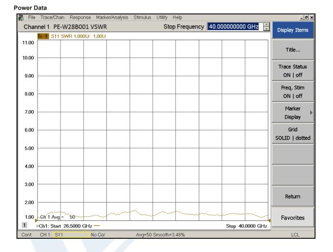
Click the following link (or enter part number in "SEARCH" on website) to obtain additional part information including price, inventory and certifications: WR-28 Instrumentation Grade Waveguide E-Bend with UG-599/U Flange Operating from 26.5 GHz to 40 GHz PE-W28B001
