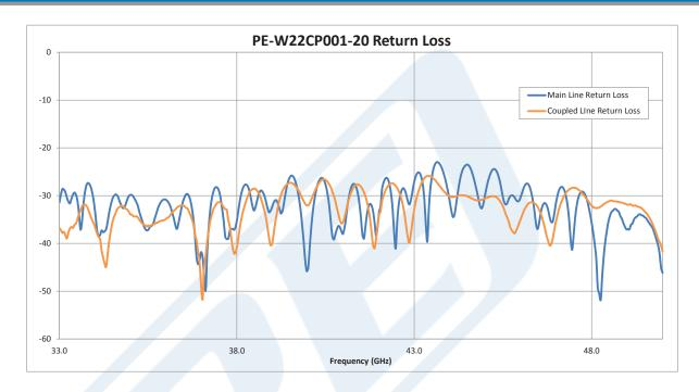
WR-22 20 dB Directional Waveguide Coupler With UG-383/U Flange and H-Plane Coupled Port From 33 GHz to 50 GHz Q Band from Pasternack Enterprises has same day shipment for domestic and International orders. Our RF, microwave and millimeter wave products maintain a 99% availability and are part of the broadest selection in the industry.
