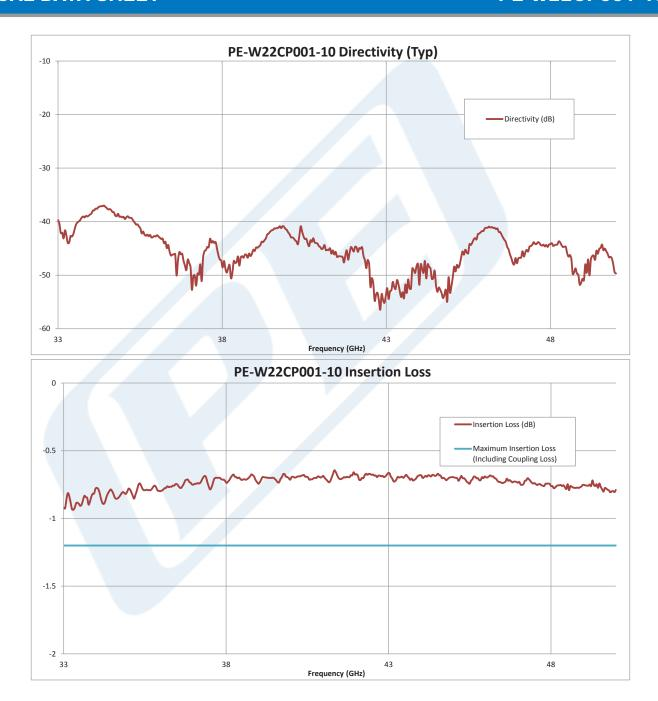
Click the following link (or enter part number in "SEARCH" on website) to obtain additional part information including price, inventory and certifications: WR-22 10 dB Directional Waveguide Coupler With UG-383/U Flange and H-Plane Coupled Port From 33 GHz to 50 GHz Q Band PE-W22CP001-10
