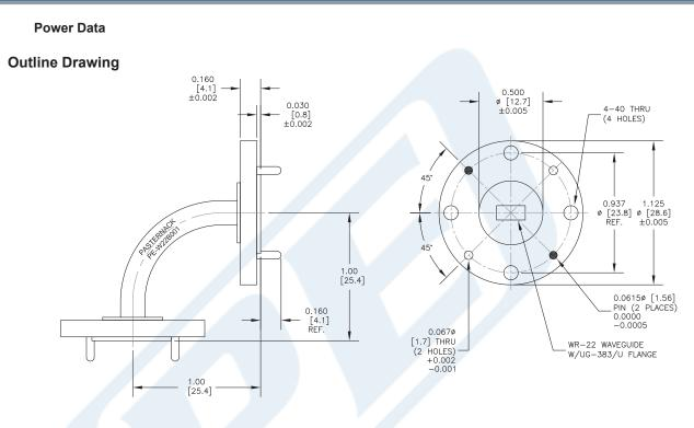
WR-22 Instrumentation Grade Waveguide E-Bend with UG-383/U Flange Operating from 33 GHz to 50 GHz from Pasternack Enterprises has same day shipment for domestic and International orders. Our RF, microwave and millimeter wave products maintain a 99% availability and are part of the broadest selection in the industry.
