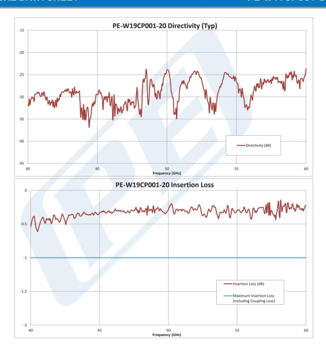
Click the following link (or enter part number in "SEARCH" on website) to obtain additional part information including price, inventory and certifications: WR-19 20 dB Directional Waveguide Coupler With UG-383/U Flange and H-Plane Coupled Port From 40 GHz to 60 GHz U Band PE-W19CP001-20
