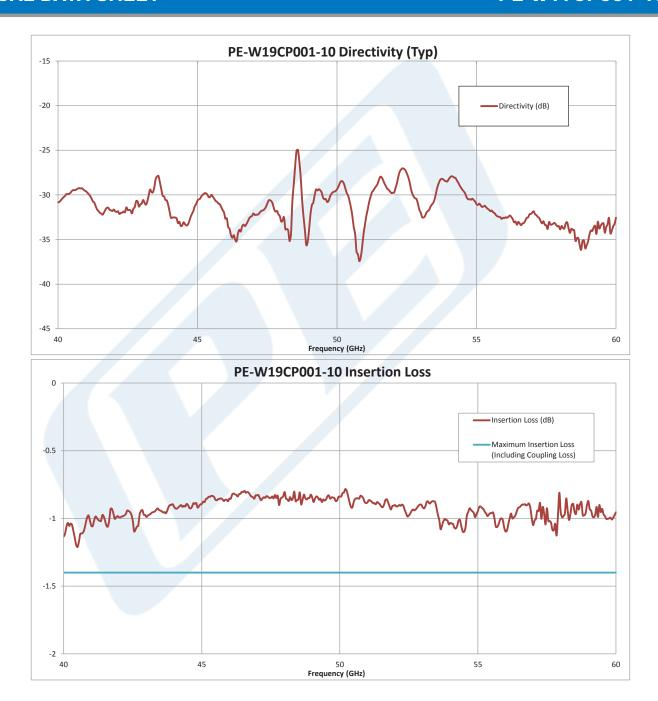
Click the following link (or enter part number in "SEARCH" on website) to obtain additional part information including price, inventory and certifications: WR-19 10 dB Directional Waveguide Coupler With UG-383/U Flange and H-Plane Coupled Port From 40 GHz to 60 GHz U Band PE-W19CP001-10
