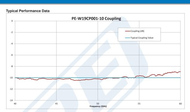
Click the following link (or enter part number in "SEARCH" on website) to obtain additional part information including price, inventory and certifications: WR-19 10 dB Directional Waveguide Coupler With UG-383/U Flange and H-Plane Coupled Port From 40 GHz to 60 GHz U Band PE-W19CP001-10
