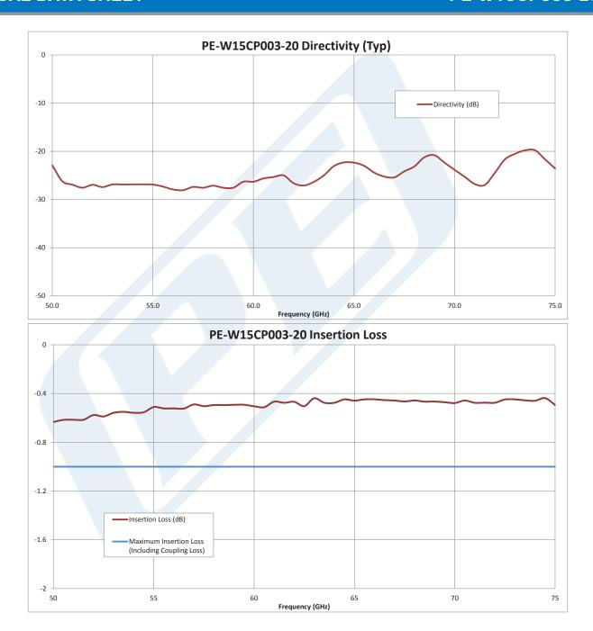
Click the following link (or enter part number in "SEARCH" on website) to obtain additional part information including price, inventory and certifications: WR-15 20 dB Directional Waveguide Broadwall Coupler, UG-385/U Round Cover Flange, E-Plane Coupled Port, 50 GHz to 75 GHz, V Band PE-W15CP003-20
