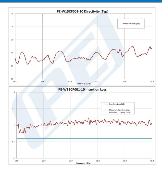
Click the following link (or enter part number in "SEARCH" on website) to obtain additional part information including price, inventory and certifications: WR-15 10 dB Directional Waveguide Coupler With UG-385/U Flange and H-Plane Coupled Port From 50 GHz to 75 GHz V Band PE-W15CP001-10
