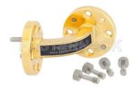
WR-15 Instrumentation Grade Waveguide E-Bend with UG-385/U Flange Operating from 50 GHz to 75 GHz
