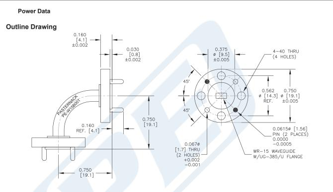
WR-15 Instrumentation Grade Waveguide E-Bend with UG-385/U Flange Operating from 50 GHz to 75 GHz from Pasternack Enterprises has same day shipment for domestic and International orders. Our RF, microwave and millimeter wave products maintain a 99% availability and are part of the broadest selection in the industry.
