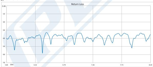
Click the following link (or enter part number in "SEARCH" on website) to obtain additional part information including price, inventory and certifications: WR-137 Twistable Flexible Waveguide 36 Inch, UG-344/U Round Cover Flange Operating From 5.85 GHz to 8.2 GHz PE-W137TF005-36
