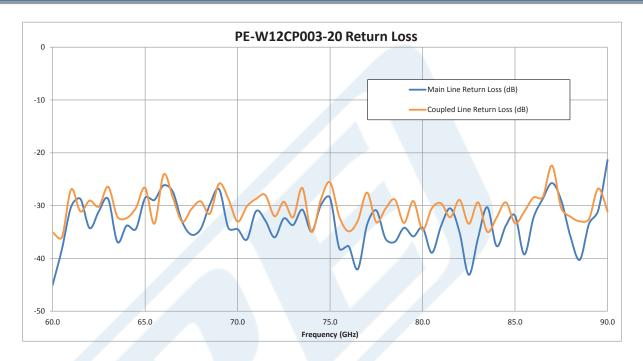
WR-12 20 dB Directional Waveguide Coupler With UG-387/U Flange and E-Plane Coupled Port From 60 GHz to 90 GHz E Band from Pasternack Enterprises has same day shipment for domestic and International orders. Our RF, microwave and millimeter wave products maintain a 99% availability and are part of the broadest selection in the industry.
