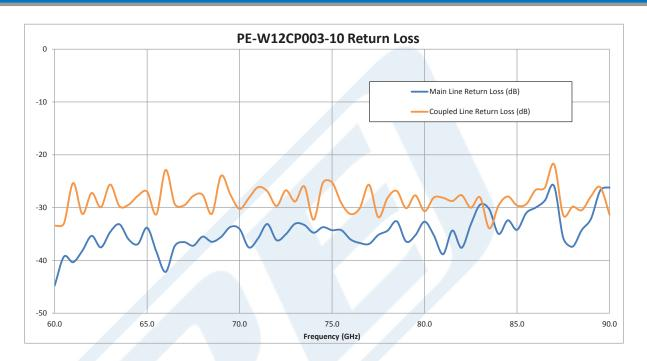
WR-12 10 dB Directional Waveguide Coupler With UG-387/U Flange and E-Plane Coupled Port From 60 GHz to 90 GHz E Band from Pasternack Enterprises has same day shipment for domestic and International orders. Our RF, microwave and millimeter wave products maintain a 99% availability and are part of the broadest selection in the industry.
