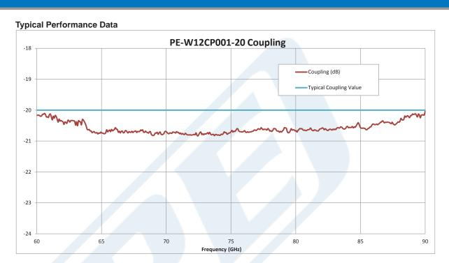
Click the following link (or enter part number in "SEARCH" on website) to obtain additional part information including price, inventory and certifications: WR-12 20 dB Directional Waveguide Coupler With UG-387/U Flange and H-Plane Coupled Port From 60 GHz to 90 GHz E Band PE-W12CP001-20
