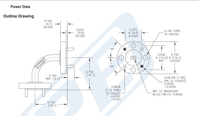
WR-12 Instrumentation Grade Waveguide E-Bend with UG-387/U Flange Operating from 60 GHz to 90 GHz from Pasternack Enterprises has same day shipment for domestic and International orders. Our RF, microwave and millimeter wave products maintain a 99% availability and are part of the broadest selection in the industry.
