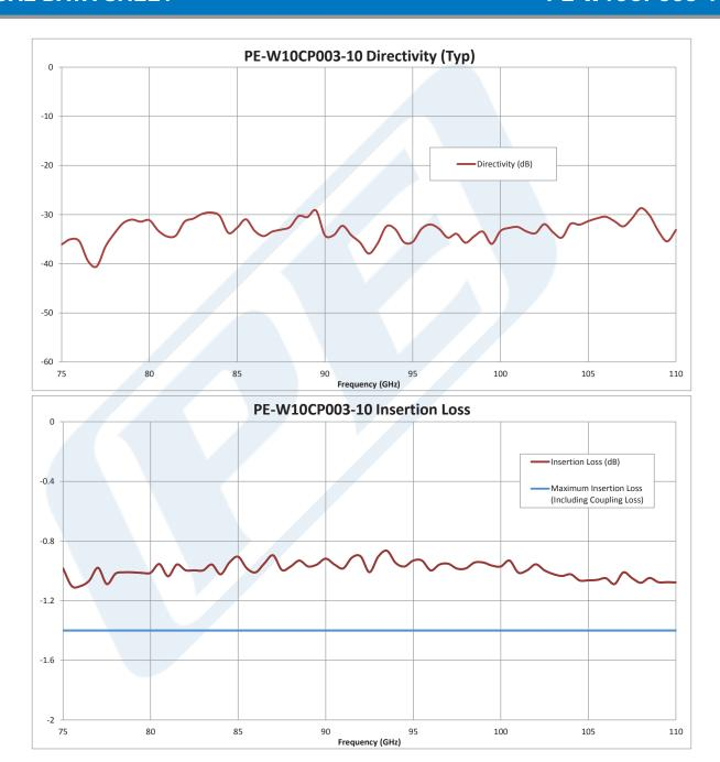
Click the following link (or enter part number in "SEARCH" on website) to obtain additional part information including price, inventory and certifications: WR-10 10 dB Directional Waveguide Coupler With UG 387/U-Mod Flange and E-Plane Coupled Port From 75 GHz to 110 GHz W Band PE-W10CP003-10
