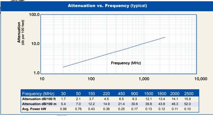
Calculate Attenuation = (0.300717) •  $\sqrt{\text{FMHz}}$  + (0.000335) • FMHz (interactive calculator available at http://www.timesmicrowave.com/cable calculators) Attenuation: VSWR=1.0; Ambient = +25°C (77°F)
