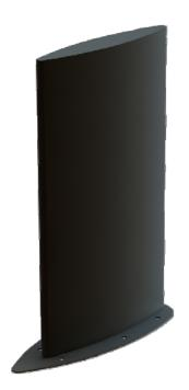
The 22-50-91 is vertically polarized, omni-directional antenna, compatible with all popular airborne radios operating within the 30 to 600 MHz frequency range. The antenna can handle upto 100 Watts of power and require no external tuning.
