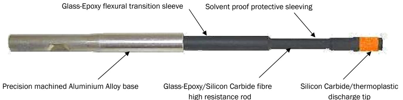
Combining Silicon Carbide and Glass-Epoxy materials, the 21-90-35 is an immensely strong, high performance Static Discharger intended for use on military aircraft operating at speeds in excess of Mach 2.
