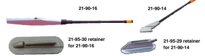
Combining Silicon Carbide and Glass-Epoxy materials, the 21-90-14 and 21-90-16 are immensely strong, high performance Static Dischargers intended for use on subsonic aircraft. With a team having over 50 years experience in the development and fabrication of aircraft static dischargers, CAL has produced an ultra reliable rugged product, specifically intended to give low initial and life cycle costs.
