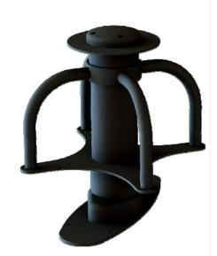
Combining highly efficient "droopy dipoles" with a wide band, line-of-sight linear element, the 21-54-49 provides Hi-Lo angle UHF Satcom from a single connector plus a separate VHF/UHF/EPLRS element in a single airborne antenna. In addition, this antenna includes an L1 stacked patch active GPS element.
