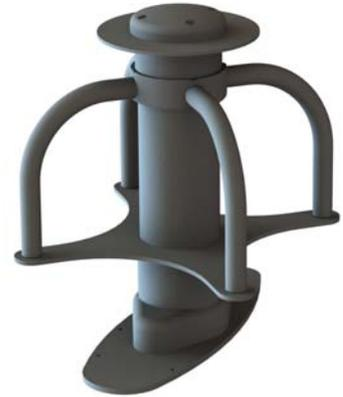
Combining highly efficient “droopy dipoles” with a wide band, line-of-sight linear element, the 21-54-46 provides Hi-Lo angle UHF Satcom from a single connector plus a separate VHF/UHF/EPLRS element in a single airborne antenna. In addition, this antenna includes an L1/L2 stacked patch active GPS element.
