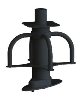
Combining highly efficient "droopy dipoles" with a wide band, line-of-sight linear element, the 21-52-46 provides Hi-Lo angle UHF Satcom from a single connector plus a separate VHF/UHF/EPLRS element in a single airborne antenna. In addition, this antenna includes a vertically polarized discone element for L-band systems such as IFF, MIDS and TACAN.
