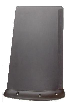
The 21-50-98 is vertically polarized, omni-directional antenna, compatible with all popular airborne radios operating within the 30 to 512 MHz frequency range. The antenna can handle 100 Watts of power, requires no external tuning and is designed as an extended frequency coverage replacement for AS3191 to operate with latest JTRS radios.
