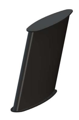
The 21-50-83 is a rugged multifunction VHF/UHF communications antenna designed for airborne applications. A high strength vertical shell houses 30 - 174 and 225 - 512MHz linear elements to be used with separate VHF & UHF line of sight "LOS" communications radios. Footprint is compatible with Collins 437S-1H and Chelton 12-437 series antennas.
