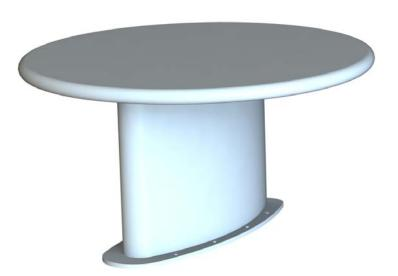
The 21-50-72 is a rugged multifunction UHF LOS plus UHF Satcom antenna designed for airborne applications. A high strength aerodynamic vertical shell houses a 225 - 450 MHz linear element that can be used for UHF line of sight "LOS" communications or UHF Satcom at low angles of elevation. This vertical shell also supports a circular horizontal disc containing a pair of cross dipoles connected to provide high angle, right hand circularly polarized UHF Satcom coverage.
