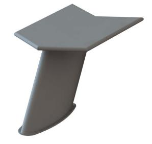
The 21-50-71-2 is a rugged multifunction VHF, UHF, C/D Band and UHF Satcom antenna designed for airborne applications. A high strength aerodynamic vertical shell houses a 30 - 1220 MHz three dimensional linear element that can be used for VHF, UHF, APC025 C/D-Band line of sight "LOS" communications or UHF Satcom at low angles of elevation.
