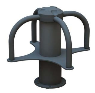
Combining highly efficient "droopy dipoles" with a wide band, line-of-sight linear element, the 21-50-61-1 provides Hi-Lo angle UHF Satcom from a single connector plus a separate VHF/UHF element in a single antenna.
