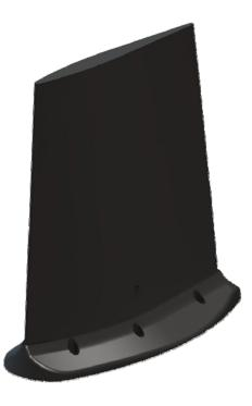
The 21-50-59 is a vertically polarized, omni-directional antenna, compatible with all airborne radios operating within the 225 to 512 MHz frequency range plus Link16, TACAN, IFF, JTIDS and other L/S-band systems.
