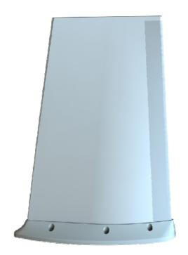
The 21-50-56-4 is a combined VHF/L-Band blade antenna suitable for use with VHF ATC and IFF systems fitted to helicopters and fixed wing aircraft operating up to Mach 0.9. Construction comprises a high strength, glass epoxy radome set into an aluminum alloy base collar with internal 'foamed-in-place' radiating, matching and filtering elements. RF design insures good azimuthal omnidirectivity and minimal interaction between VHF and IFF-SSR elevation patterns.
