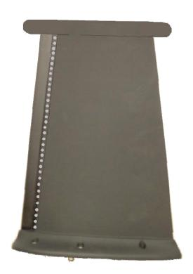
The 21-50-51 is a vertically polarized, omni-directional antenna, compatible with all popular airborne radios operating within the 30 to 600 MHz frequency range. These antennas can handle 30 Watts of power and require no external tuning.
