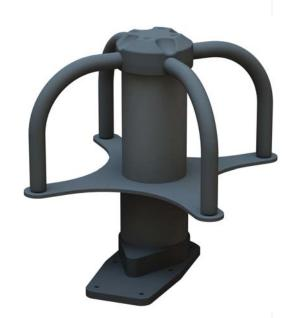
Combining highly efficient "droopy dipoles" with a wide band, line-of-sight linear element, the 21-50-48 provides Hi-Lo angle UHF Satcom from a single connector plus a separate VHF/UHF/EPLRS element in a single airborne antenna.
