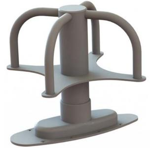
Combining highly efficient "droopy dipoles" with a wide band, line-of-sight linear element, the 21-50-46 provides Hi-Lo angle UHF Satcom from a single connector plus a separate VHF/UHF/EPLRS element in a single airborne antenna.
