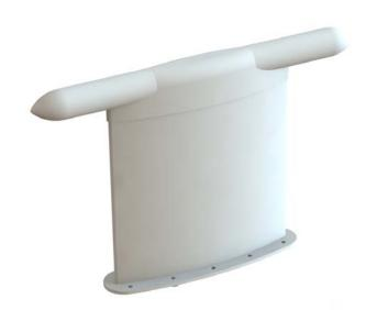
The 21-50-334 is a vertically polarized, omni-directional antenna, compatible with all popular airborne radios operating within the 29.5 to 960 MHZ frequency range. This antenna can handle up to 25 Watts of power and requires no external tuning.
