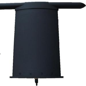
The 21-50-32 is a vertically polarized, omni-directional antenna, compatible with all popular airborne radios operating within the 30 to 600 MHZ frequency range. This antenna can handle up to 100 Watts of power and requires no external tuning.
